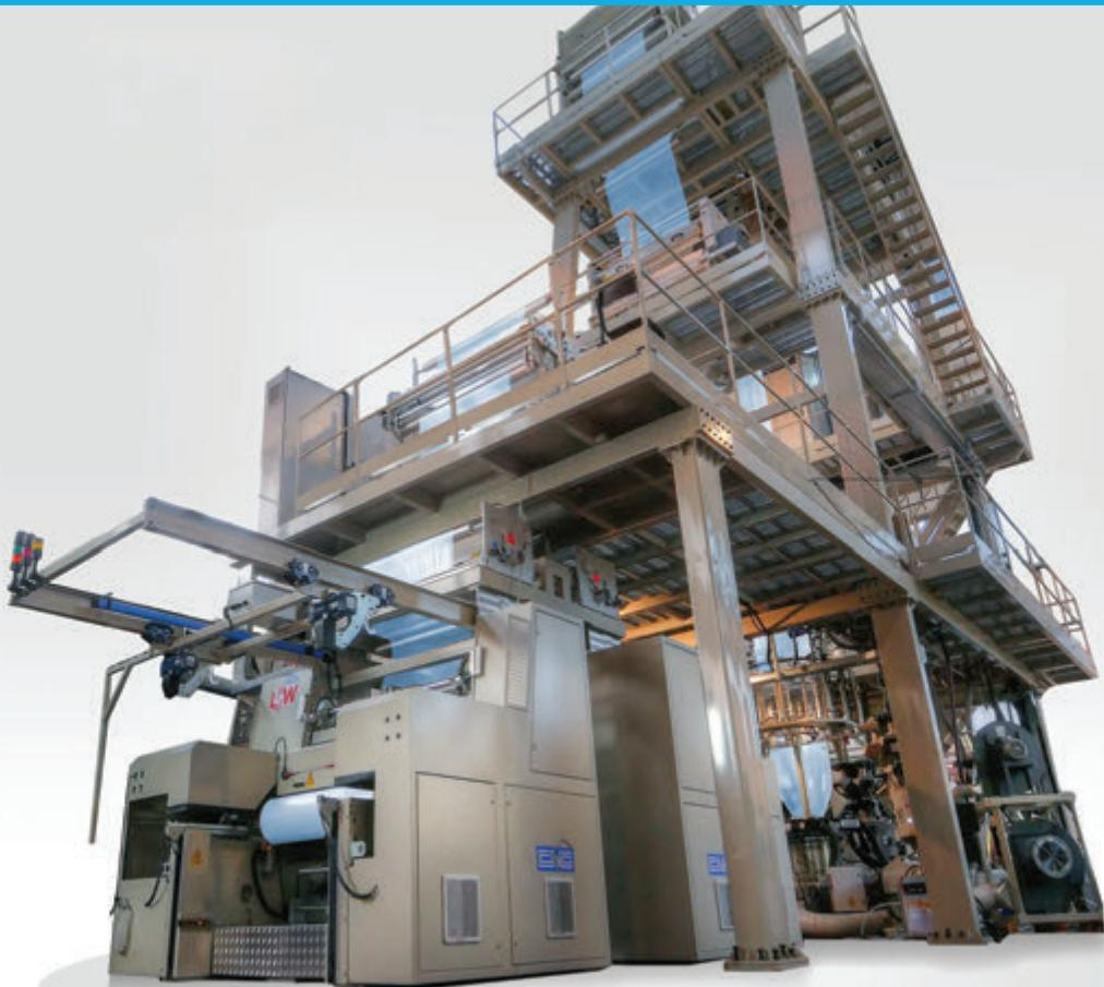
The development of the CMG know-how in the coextrusion process has enabled us to offer to our Customers plants for the production of multilayers film by processing both conventional polyolefins and materials for getting the barrier effect.
