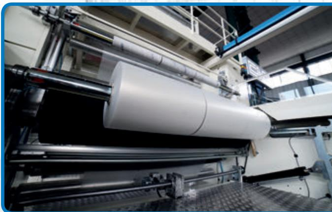
New LSW: Top-of-the-range winder for blown film extrusion lines
